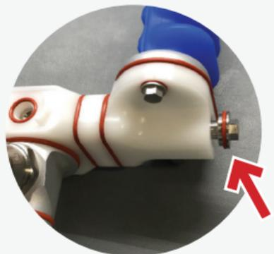
*Note:* Use the Tie Rod and spacer chart (located on the right panel of this guide) to identify which tie rod is best for your gripper. We recommend Anti-Seize gel onto the Tie Rod before M4 Hex Nut is installed.
